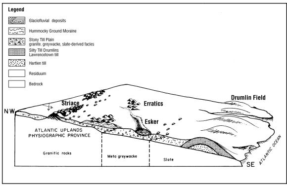
Figure T3.4.1: Cross section of the Quaternary deposits of the Atlantic coast of Nova Scotia.1
