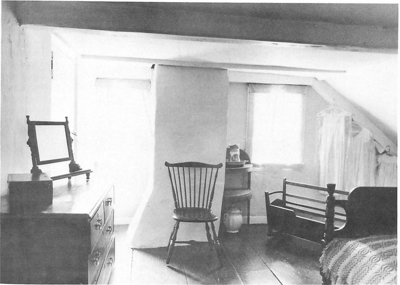
Bedroom 1 looking west. The structural frame and chimney are visible with the 2 flues from the Office and Parlour gathering into one to eject smoke close to the peak of the roof.
