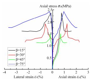
Fig. 2 Typical stress-strain curves of columnar jointed rock mass specimens under uniaxial compression tests
