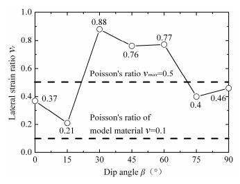
Fig. 3 Variation of lateral strain ratio  $v_r$ , vs dip angle  $\beta$
