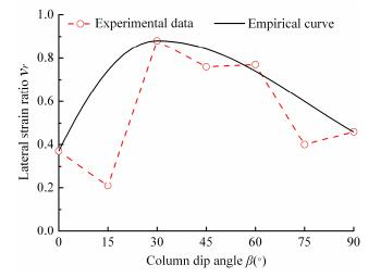
Fig. 5 Lateral strain ratio  $v_r$  vs dip angle  $\beta$
