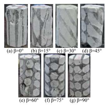
Fig. 4 Typical failure modes of columnar jointed rock mass specimens
