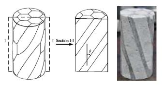
Fig. 1 Sketches of columnar jointed rock mass specimens
