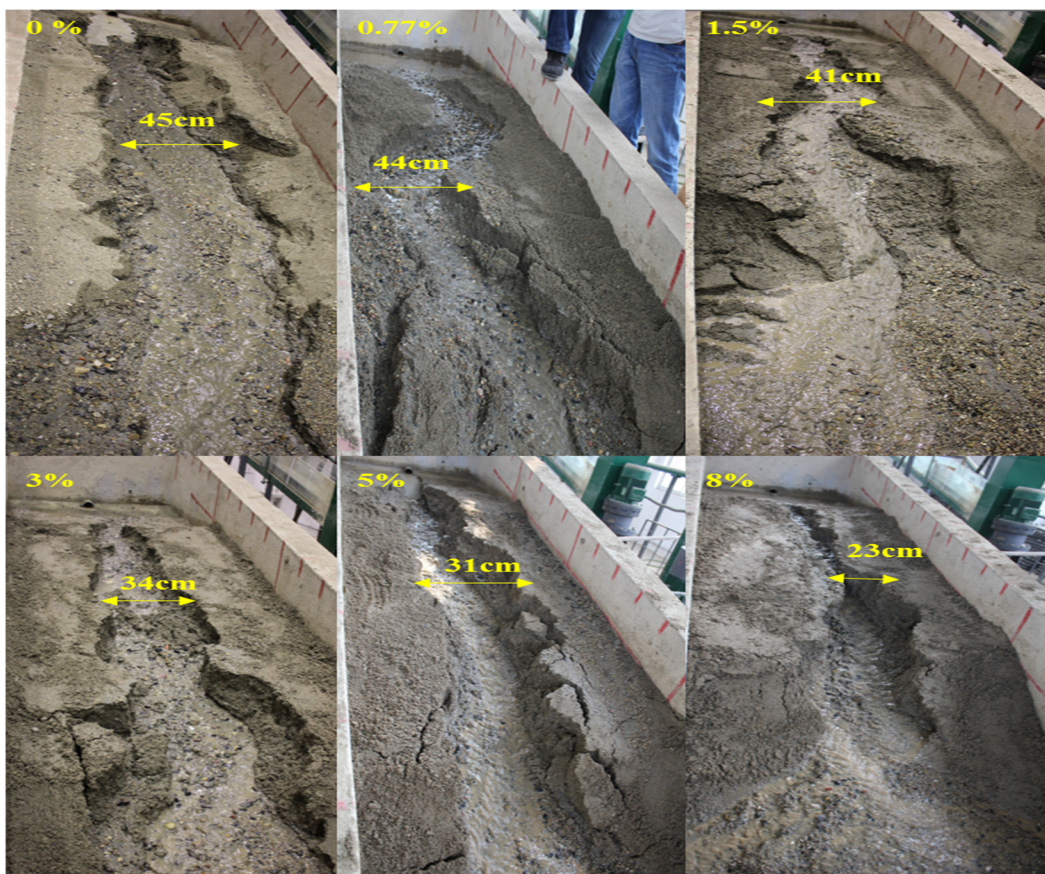
Figure 14. The effect of clay content on erosion, higher clay contents result in narrower channels. The measurement position is located in the middle of the deposition, d_{50} = 1.8 mm, C_u = 29 , surface slope 10^\circ
