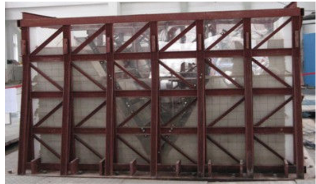
Figure 1. The slope model before the test (the left part is the Limestone slope and the right part is the Mudstone slope)
