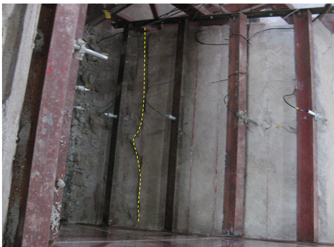
Figure 9. Cracks in the mudstone slope model: the toe of slope and the crest of slope
