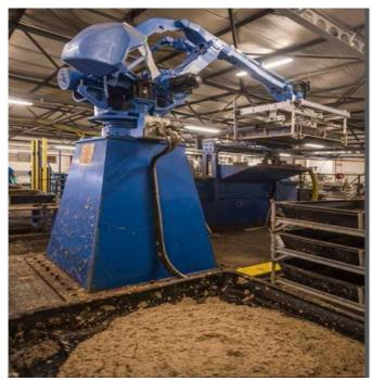
Figure 5. Robotic co-ordination at the twenty-four-hour canteen. Larvae lunch is pumped from two silos in the waste processing plant to meet the larvae recyclers who initiate the bio-conversion process. Photo: Charlie Drew.
