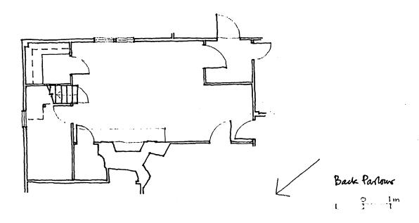
Back Parlour Plan 1949. Restored as much as possible to its original kitchen appearance of pre-1792, the room is now a complex space to study. Partitions and cupboards were relocated in 1949 when the stair was returned to its front position.
