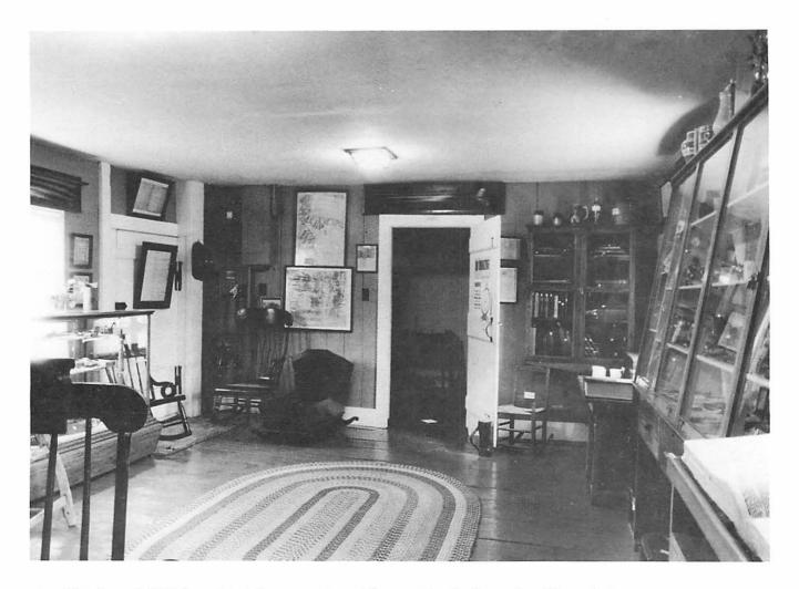
The Kitchen Addition looking north. The central door leading into the main house was installed during the 1949 alterations, replacing two separate doors. At the left is an external door and beneath the crib is a trap door giving access to the cellar.
