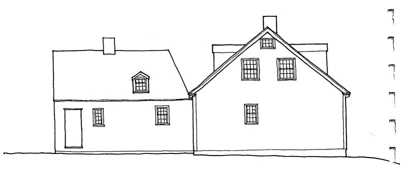
The East Elevation of 1792 clearly defines the addition of the kitchen. By holding the roof of the addition back from the original roof, the south-facing dormer could be maintained.
