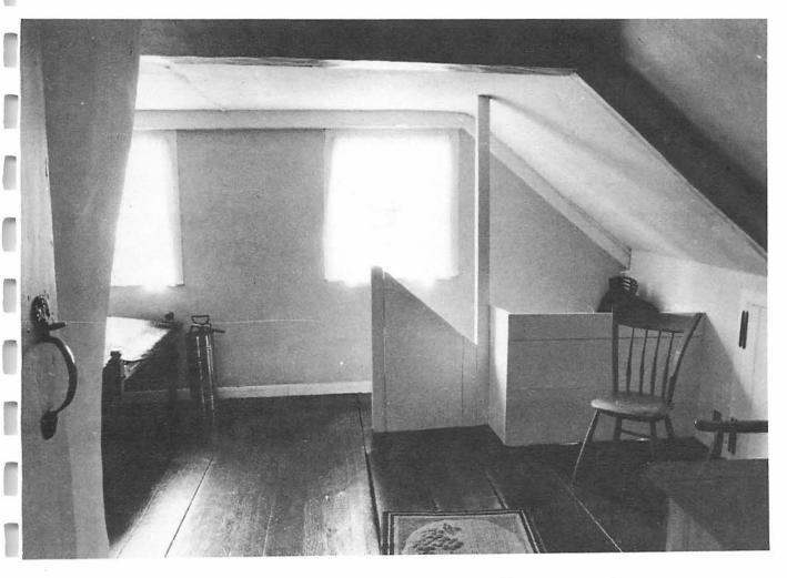
Bedroom 3 looking east. Marks in the end wall and ceiling suggest a partition has been removed, which would have divided this room into two rooms, each with a window.
