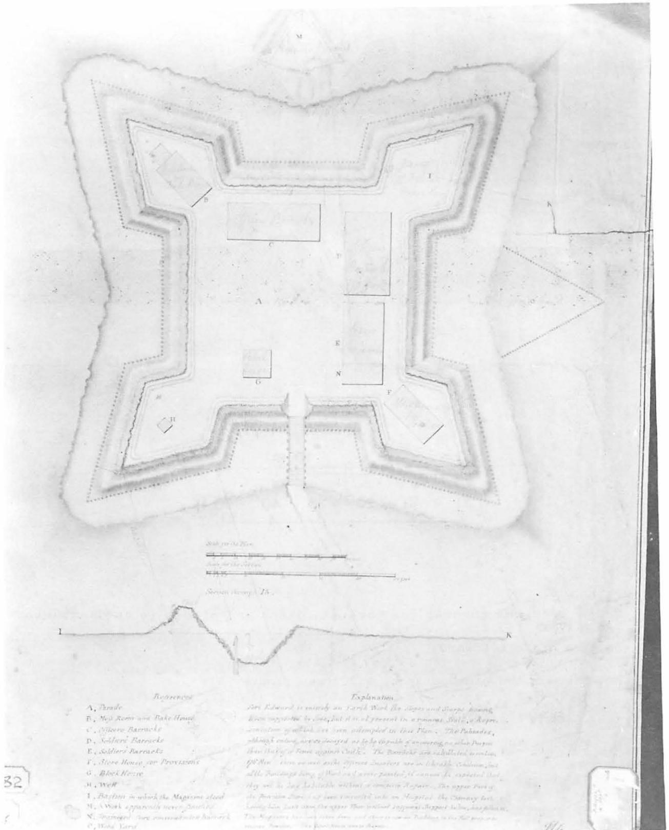
6. A plan of Fort Edward by W. Fenwick, 1799-1800 (Public Archives of Nova Scotia). The configuration of the palisade and ditch is similar to that in the 1779 plan. The cross-section (see Figure: 7B) shows the deterioration of the earthworks by the end of the 18th century. The palisade is described as "so decayed as to be capable of answering no other Purpose than that of a Fence against Cattle."
