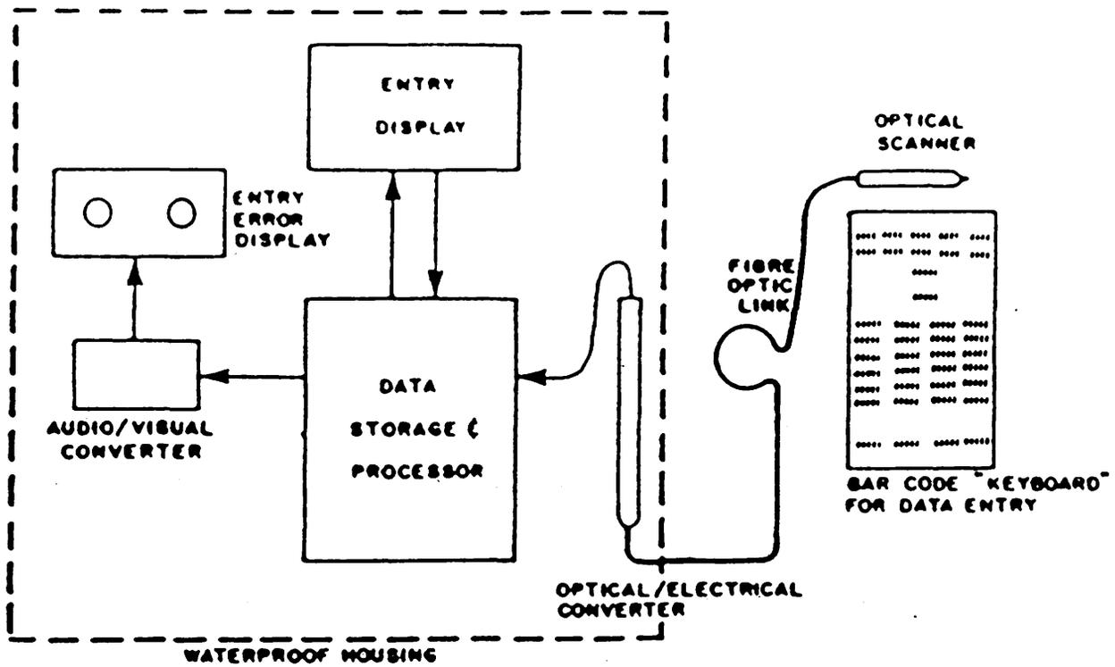
Figure 1. Component diagram of the diver-operated computer.
