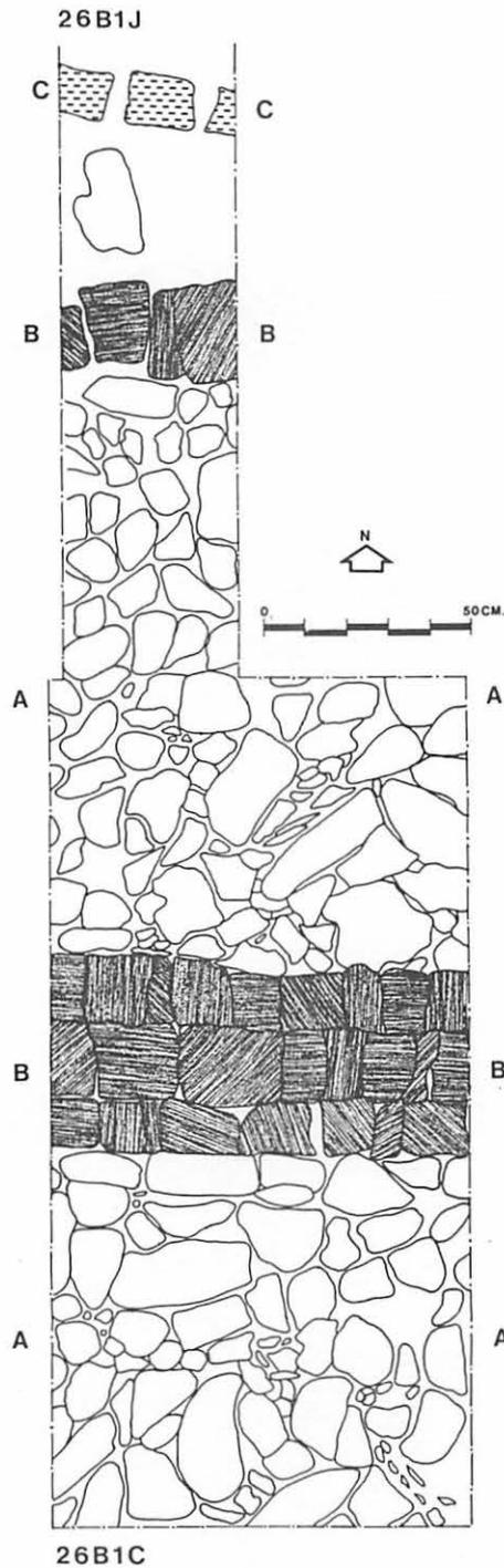
14. 26B1C,J: Plan of cobblestone pavement in front of soldiers' barracks, with drain and edging of cut quartz sandstone.
