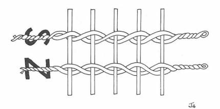
Figure 4. Diagram of the S- and Z-twists used in twining and cordage.
