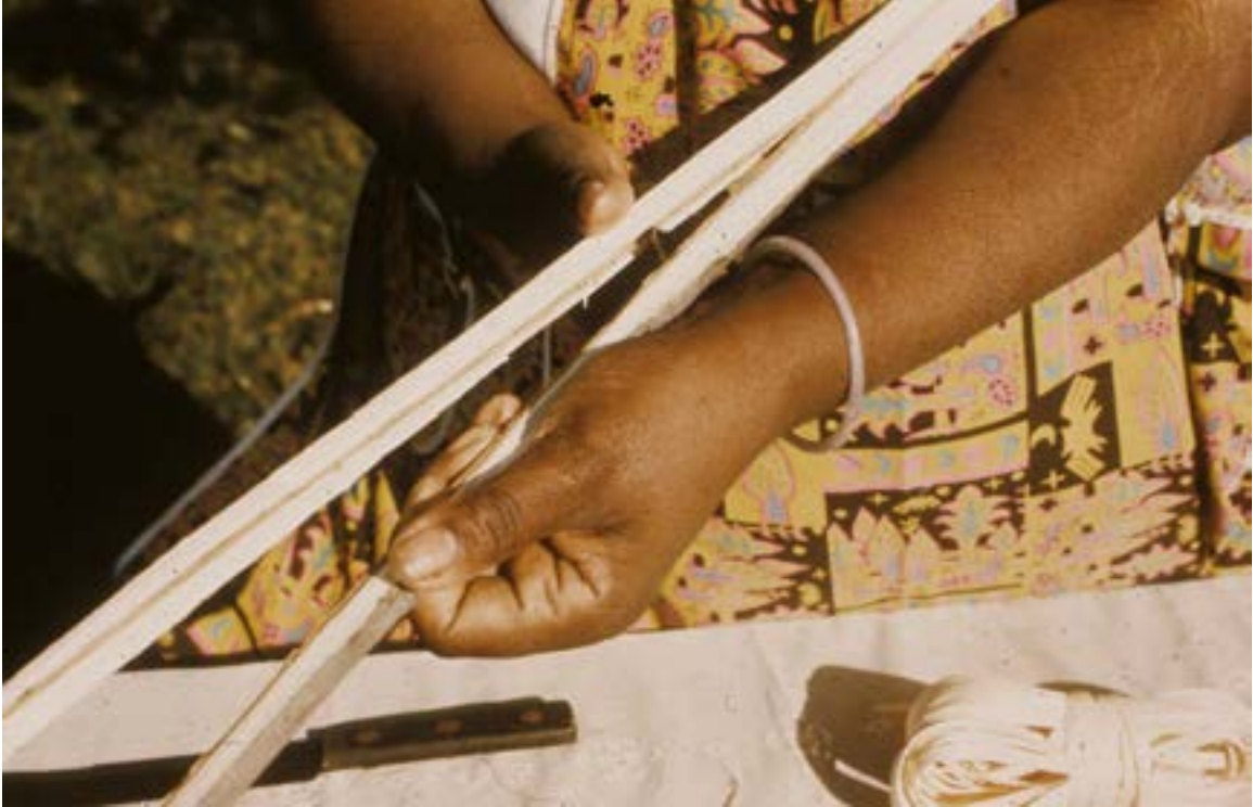
Figure 48. Split the quartered wood into two equal portions, bracing the end against the body and pulling away with the left hand. Nova Scotia Museum, History Collection.
