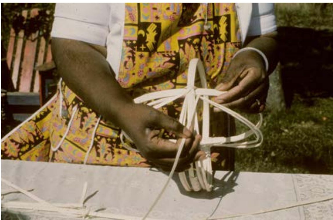
Figure 72. Insert a split between rim and uppermost pair of ribs. Nova Scotia Museum, History Collection.
