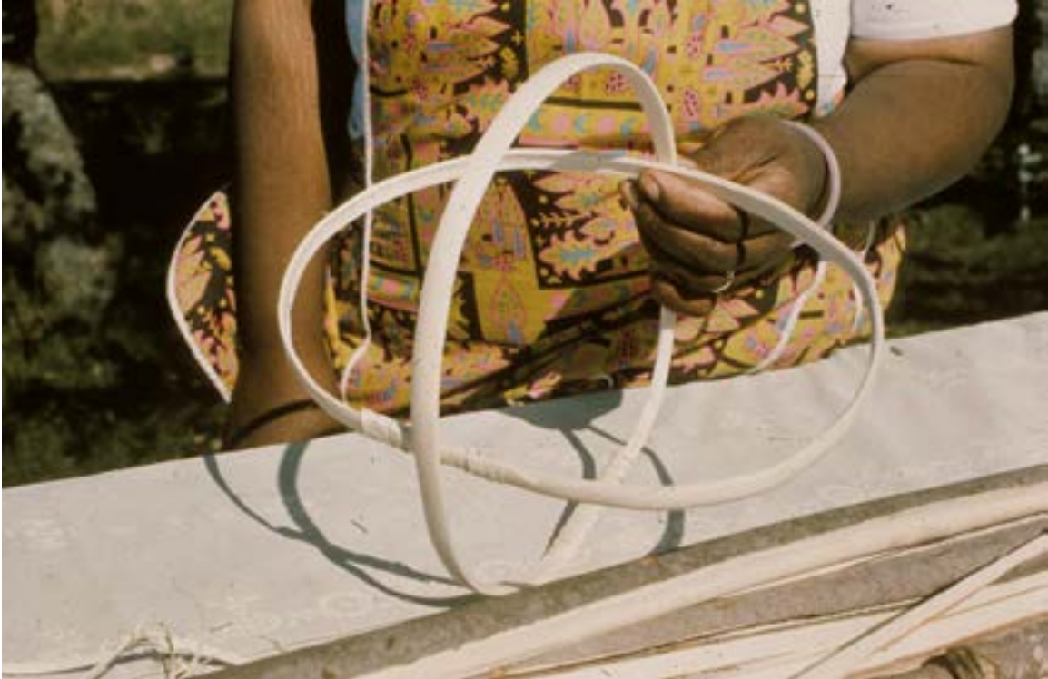
Figure 62. Insert rim circle inside the handle circle, at right angles. Nova Scotia Museum, History Collection.
