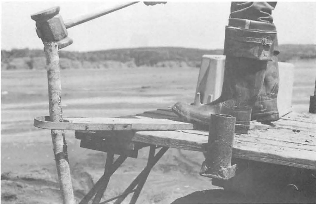
*Figure 49. Gerald's gadget for holding the stakes in place while pounding.*
