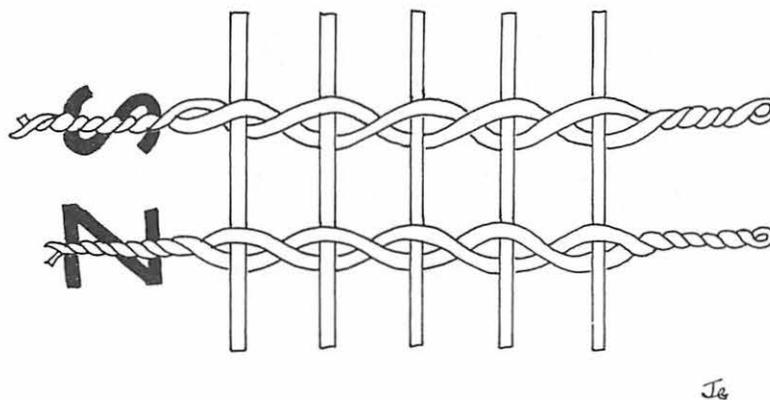
Figure 4. Diagram of the S- and Z-twists used in twining and cordage.
