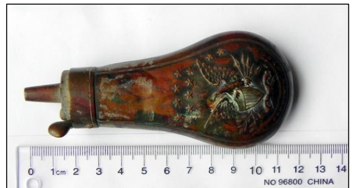
Plate 1: Brass gunpowder flask for a Colt pistol, model 1849, found in Tusket Falls.
