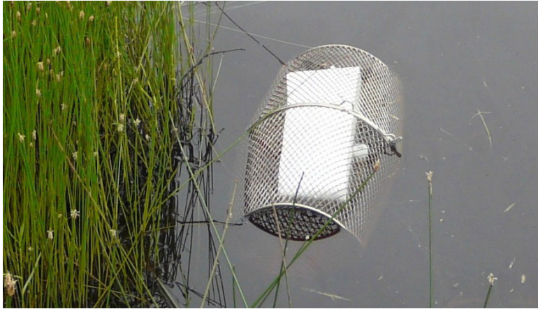
Fig 1 A light-baited trap set in a wetland pool. Note the end of the glowstick to the right of the Styrofoam® float.
