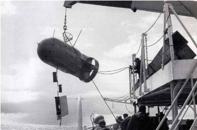
Fig 4 Deploying a current meter mooring the Drake Passage.
